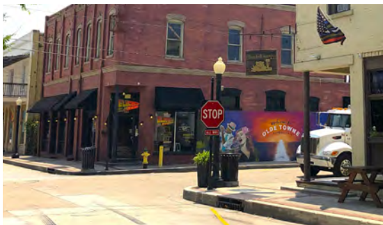
The intersection of Cousin and Carey Streets is a key one for Olde Towne, but it lacks both “pedestrian bulbs” and ADA-compliant ramps for the mobility challenged.
