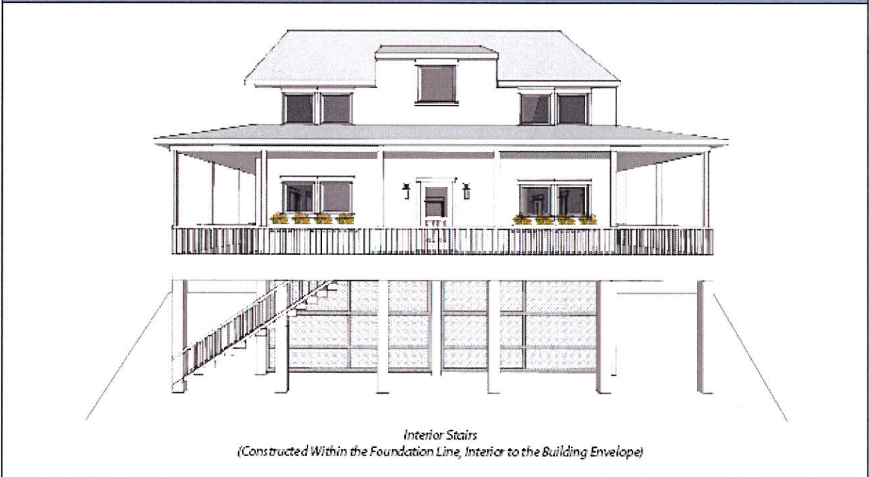
Figure 13.202.4 Illustration of Covered Walkway and Interior Stairs
