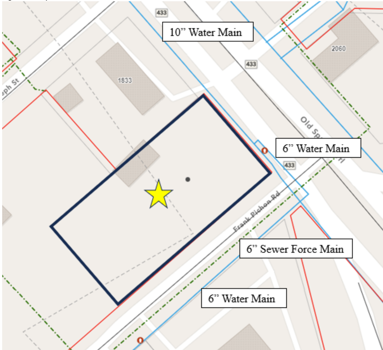
Figure 5. City water and sewer
