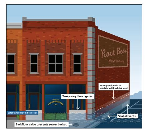
"Dry floodproofing" is intended to keep all flood waters out of a building. The graphic at left is from a document entitled "Guidelines on Flood Adaptation for Rehabilitating Historic Buildings" prepared for the National Park Service (NPS) in 2019. This approach includes waterproofing walls, sealing openings, and installing backflow prevention devices. Any waterproof coatings should be carefully researched before applying them to historic wall surfaces and materials.
