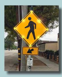
This flashing signage is activated by a button pushed by pedestrians. That same button can trigger a red light when a traffic signal is also installed at the intersection. This treatment can occur on both Front Street and Fremaux Avenue.
